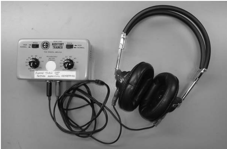
Figure 8.7 A self-contained (auditory trainer) amplification system.
